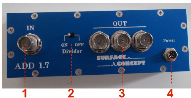
Figure 1: Connector Layout of ADD 1.7
