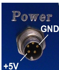
Figure 3: Pin configuration of 5pin power socket of ADD 1.7.
